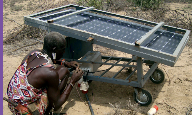
A farmer fixing his portable solar system that is used for water pumping and lighting ©Noah Lusaka
