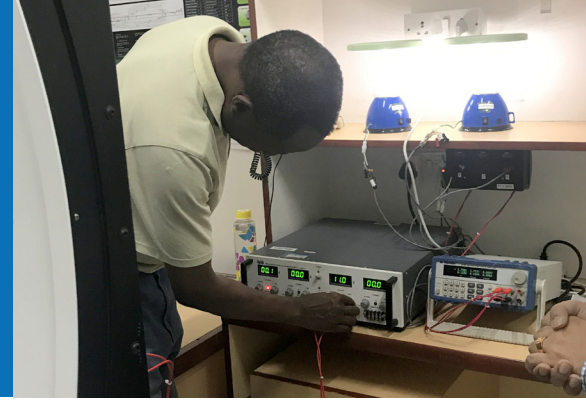
A lumen performance testing experiment at the TERI University laboratory in New Delhi, India ©KIRDI
